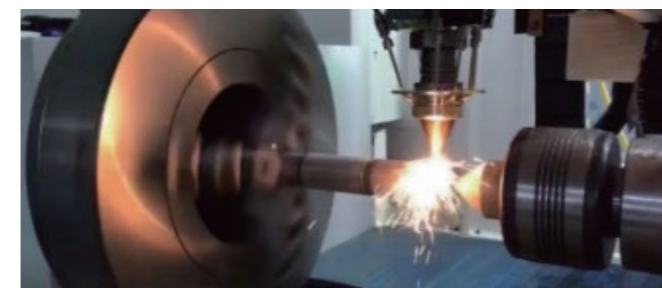
Figure 3-3: Repairing Worn Parts Using Laser Additive Manufacturing Technology
