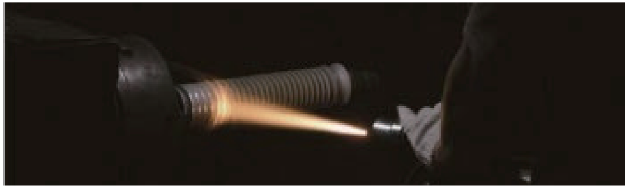
Figure 3-4: Repairing Worn Parts Using Plasma Spraying Technology
