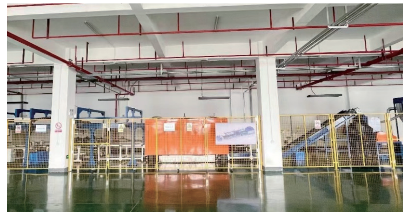
Figure 8-5: Demonstration Line for Physical Disassembly of Modules (20MW/a)
