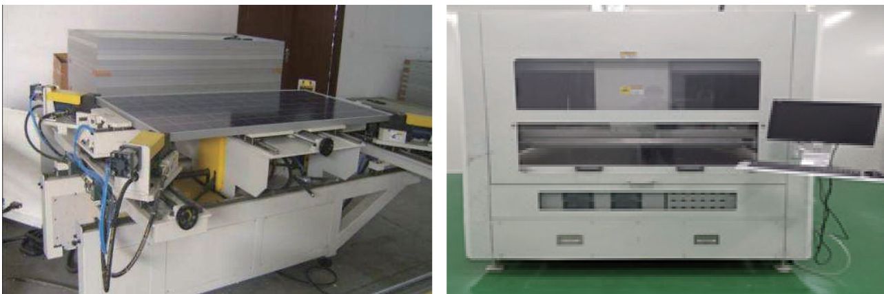
Figure 8-4: Automatic Frame Dismantling System and Automatic Backsheet Dismantling Tunnel Kiln
