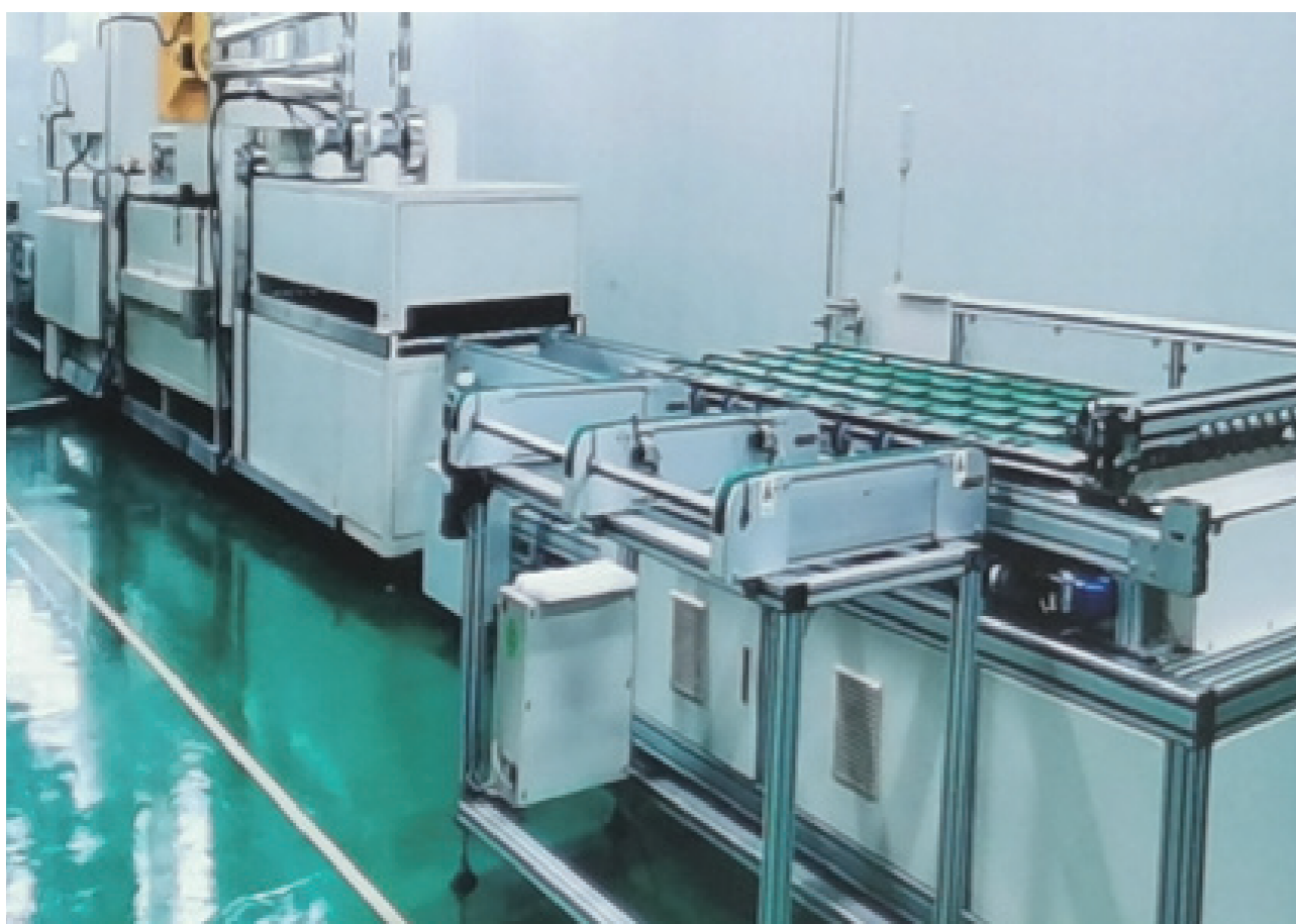
Figure 8-6. Demonstration Line for Chemical Method Silicon PV Module Recycling (12 MW/year)
