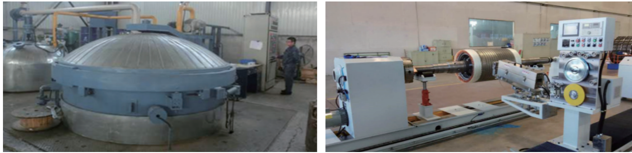
Figure 3-2: Remanufacturing of Generators
